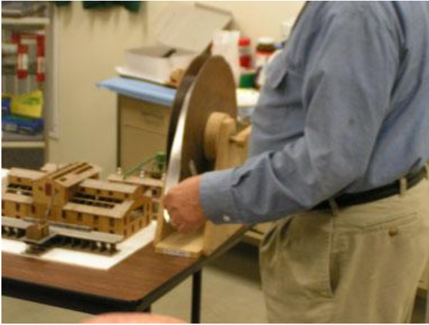
Duncan explains the manufacturing technique of making HO scale aluminum roofing.
